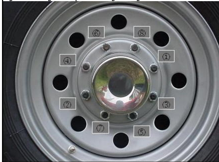
Figure 7-1 Lug nut sequence of tightening
