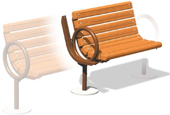
Model BE43/CW-3IB34 3 Ft. Embedded Mount Bench Extension with Brown Powder Coat Frames and Indonesian Balau Wood 3" x 4" Timbers. (Shown with Model B43/CW-3IB34 Bench.)
