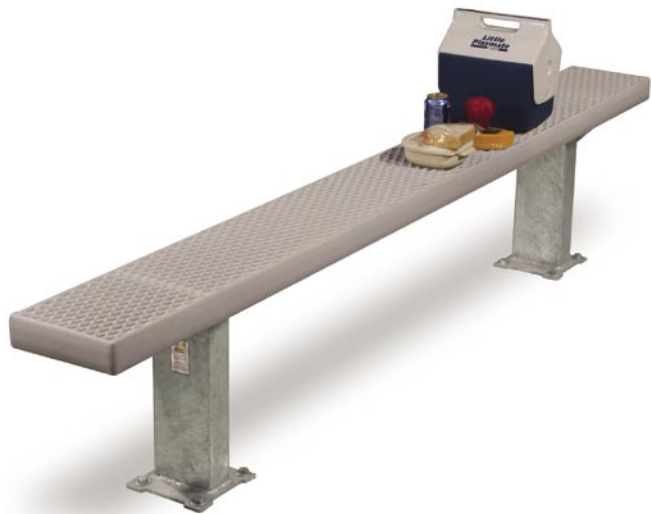
Model APB/P/G-8VA10 Surface Mount Bench with Hot Dip Galvanized Frames, 8 Ft. long with 10" wide Gray Plastisol Coated V-Type Expanded Steel seat. Shown with optional base plate for surface mounting
